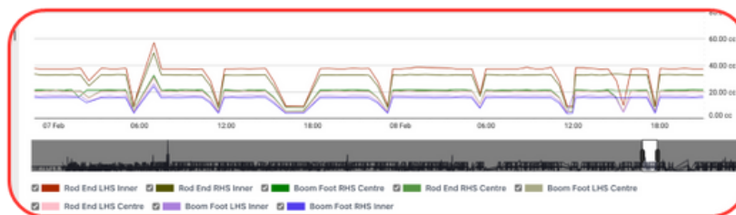
Figure 1 - Healthy lube system - consistent trends across injectors.
