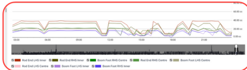
Figure 2 - Bypassing injector causing inconsistent trends across the system.
