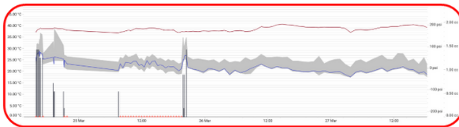
Figure 2 - Boom foot LHS showing a lack of grease applied – the same trend across multiple points
