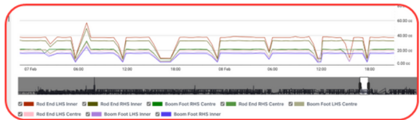
Figure 4 - Healthy lube system - consistent trends across injectors.
