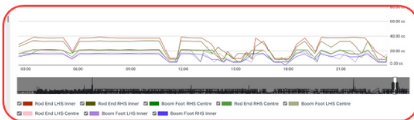
Figure 5 - Bypassing injector causing inconsistent trends across the system.
