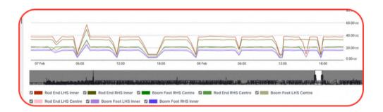
The data below shows the exact moment that an injector on the swing box (not directly monitored by Endpoints) started bypassing, the **system showed chaotic data trends** among the monitored endpoints, **enabling the identification of the issue and subsequent maintenance actions** to restore the system's consistency and health.
