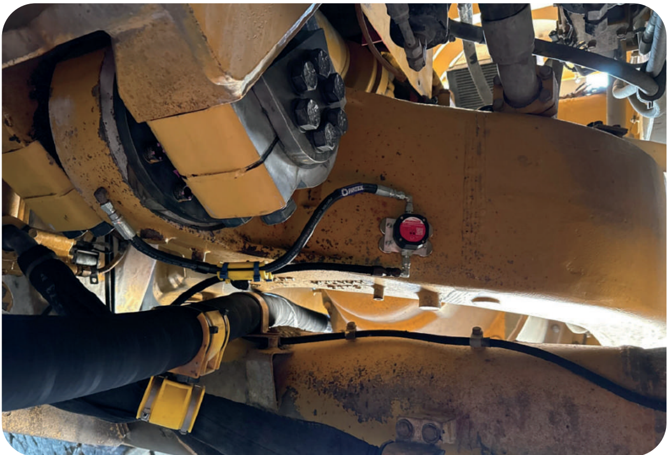
Endpoint Low Flow monitoring the A-frame bearing
