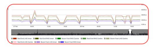
The data below shows the exact moment that an injector on the swing box (not directly monitored by Endpoints) started bypassing, the **system showed chaotic data trends** among the monitored endpoints, **enabling the identification of the issue and subsequent maintenance actions** to restore the system's consistency and health.
